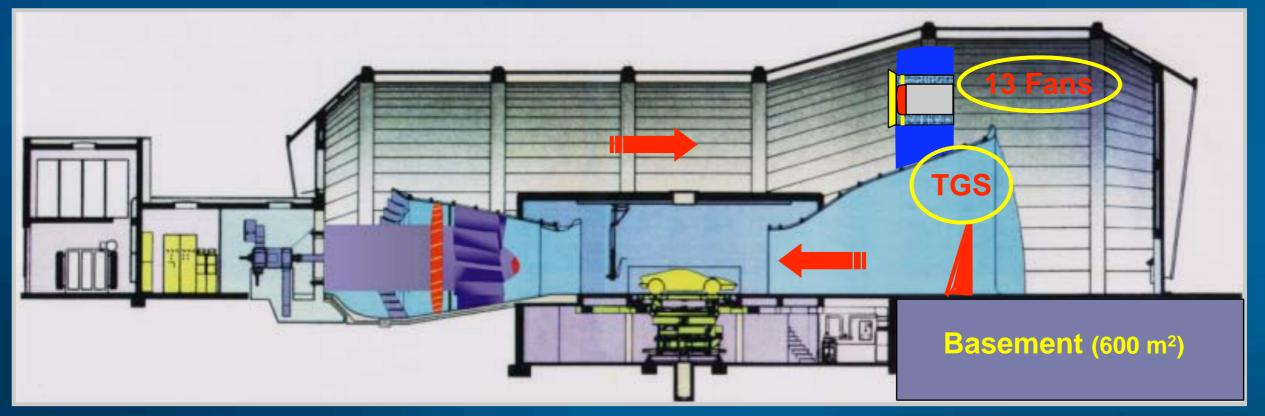
**Jet Section** Flow Max Velocity Background Noise Level : 68 dBA at V = 100 Km/h **Turbulence Intensity**
