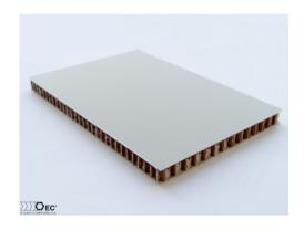
Flooring panel with 1,5 / 1,0 mm aluminum skins and Nomex core ECA-I 4.8-96, panel weight of 8,8 kg / m<sup>2</sup>, Rw = 30 dB (ISO 717-1)
