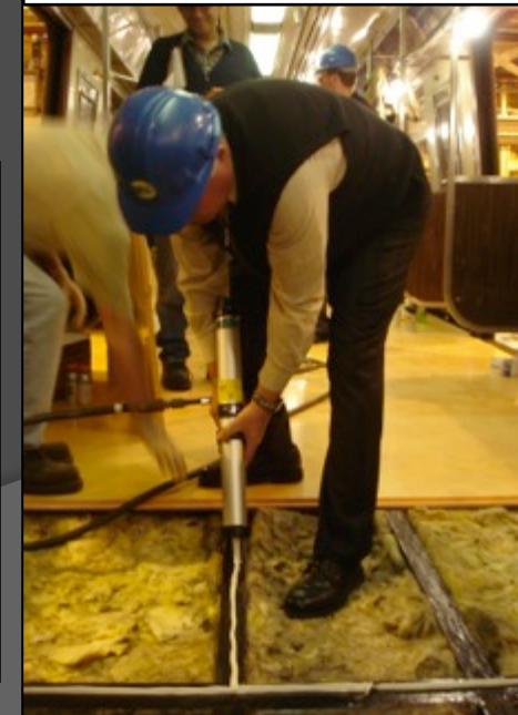
Moisture cure urethane adhesive being applied to underframe. Pneumatic gun dispenser with adhesive cartridges.
