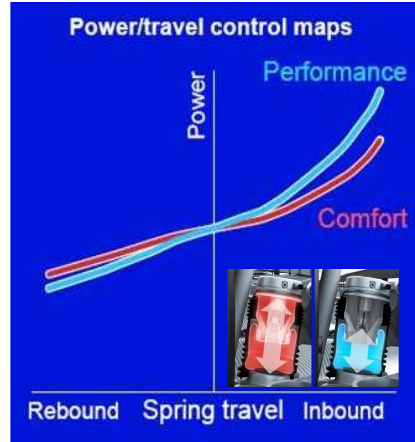
fig. 2: variation of spring rate
