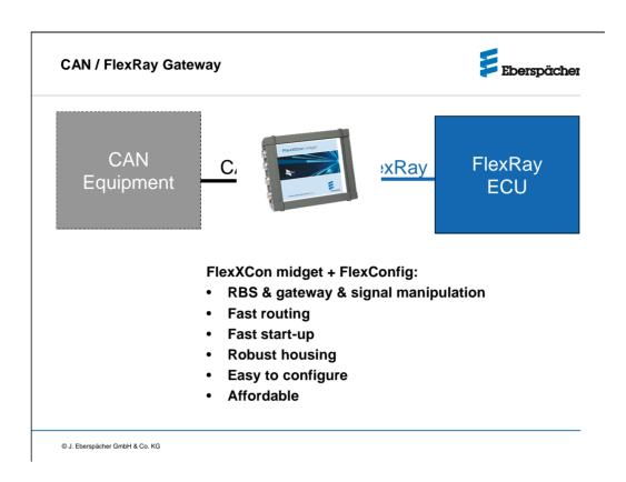
The FlexXCon family offers a hardware platform for typical applications in the networking environment. These include gateways between different bus systems, remaining bus simulation, signal manipulation and rapid prototyping. Eberspächer Electronics offers suitable products for different performance classes and uses.
