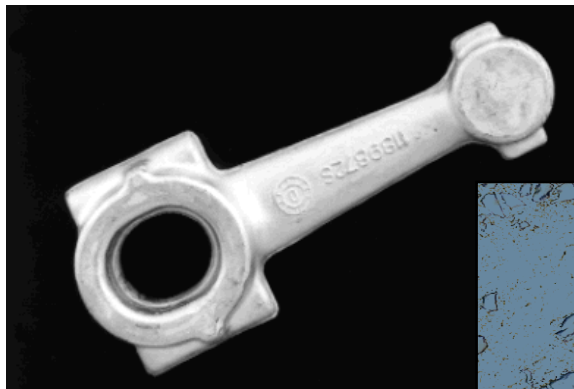
Piston, ZC71/SiC/12p ; microstructure after forging
