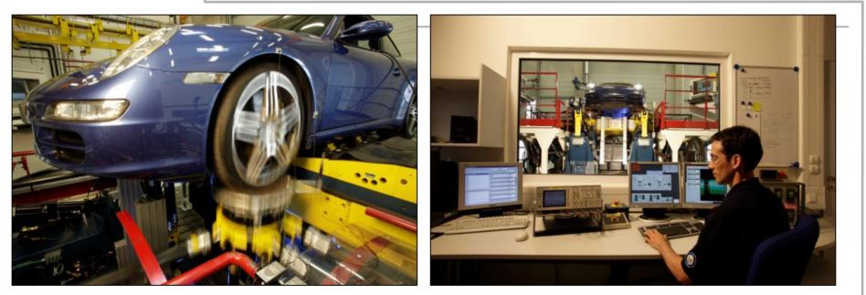
Force and displacement controlled, 2 x 16 channel 3D optical Krypton measurement device + further measurement device
