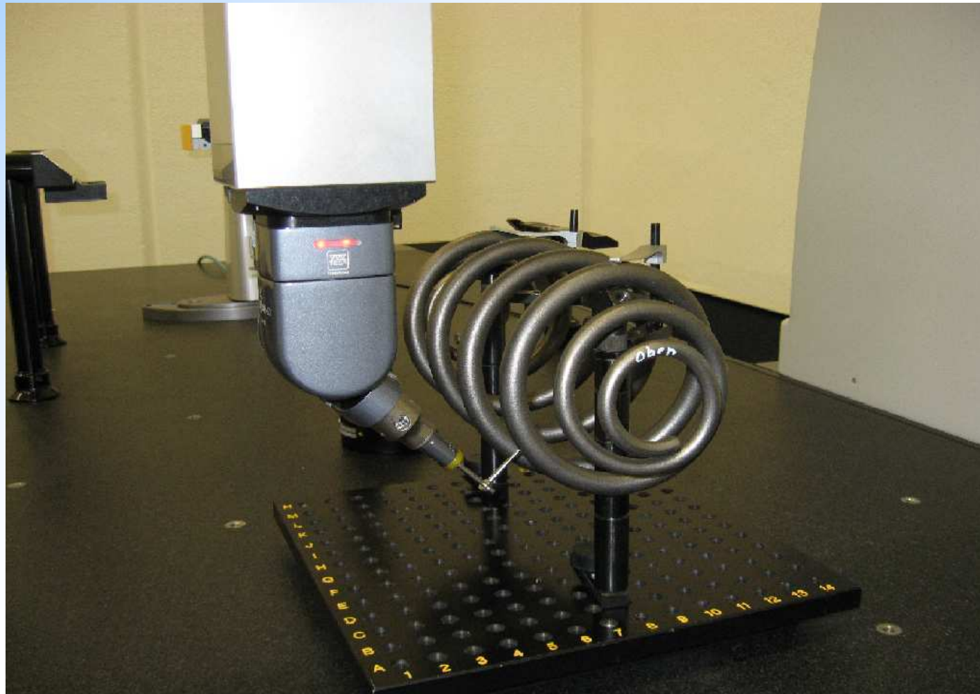
Capturing geometry data of the real spring, feedback into FEM
