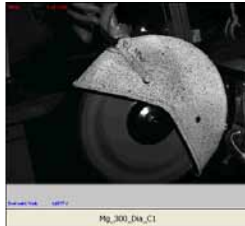
Vibration meas. on manually operated tool (friction saw) (large rigid body movement)
