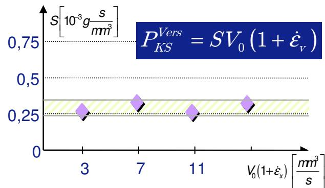
Power from plastic deformation 6-20kHz
