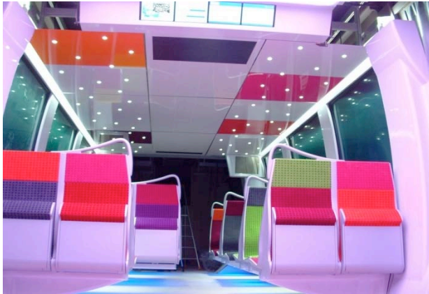
SNCF-NAT The first interior to utilise LEDs as the sole source of illumination.
