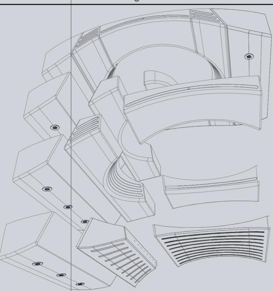
the wide variety of paneling modules enables different combinations to be used to cover the door drives and to create the most diverse interior ambiances
