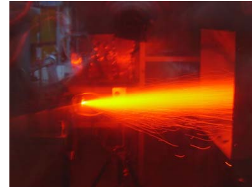
Arc wire spraying with a GTV sparc 400
