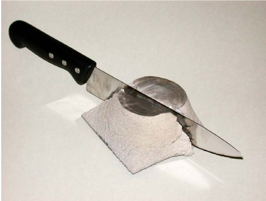
Arc wire sprayed AISi6 billet rod heated into the semi-solid state and cut easily by a kitchen knife
