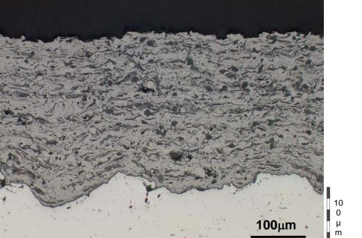
Typical MMC coating (F2056) for heavy duty Diesel engines with HV = 500
