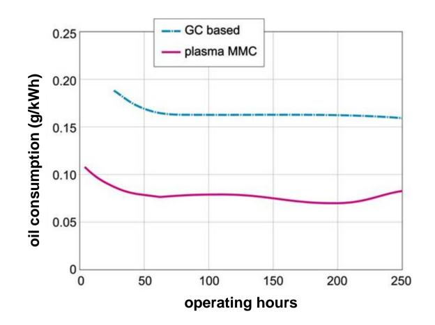
Test results prove that the plasma coating reduces the oil consumption by a factor of two
