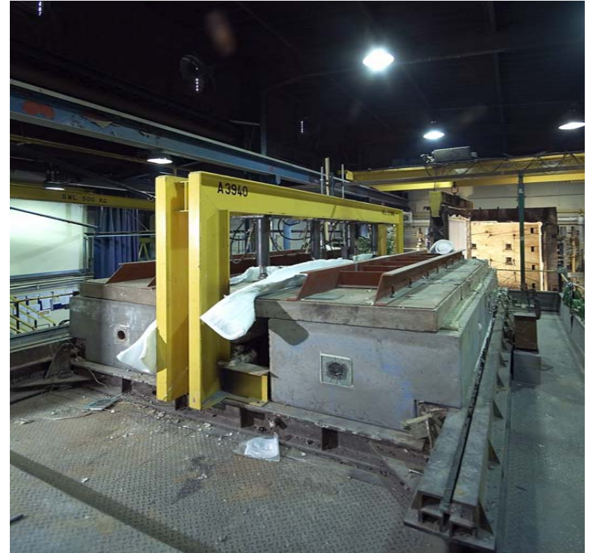
EN 1365-2 Under floor fire to passenger area
