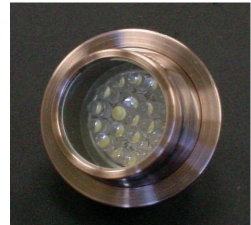
2006 - 25 LEDs - ~7fc intensity
