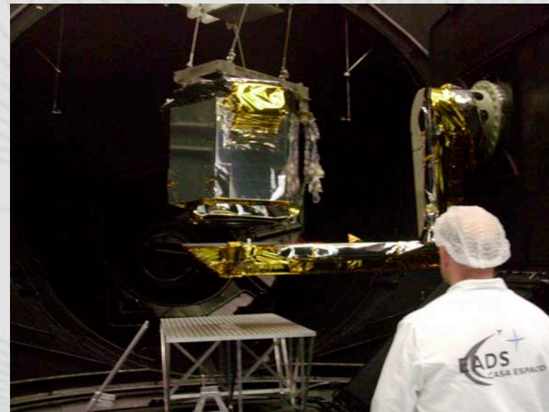
Installing the PLM on the support arm
