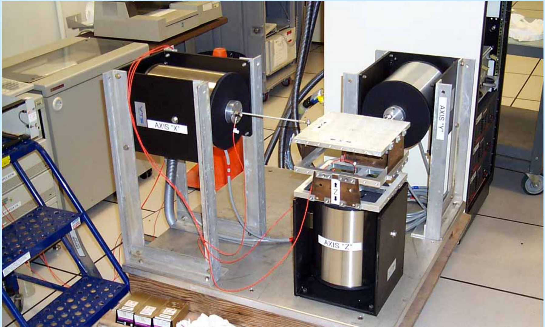
Figure 16-9 Three-shaker 3DoF concept
