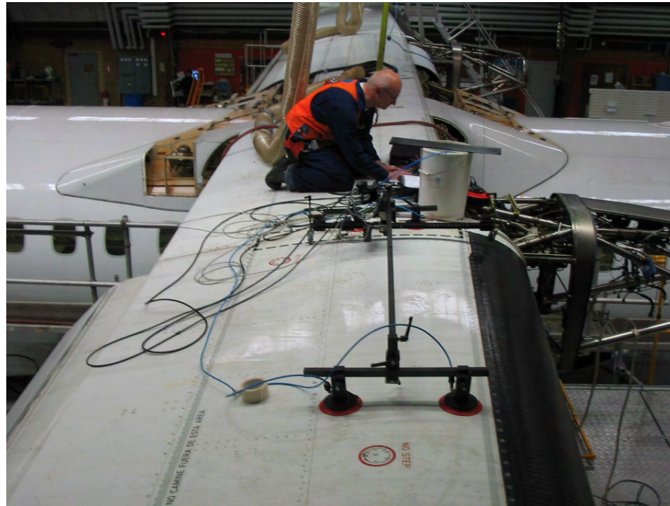
FORCE Track Scanner in operation on an ATR72 aircraft during in-service inspection (MRO) at Cimber Air Maintenance Centre
