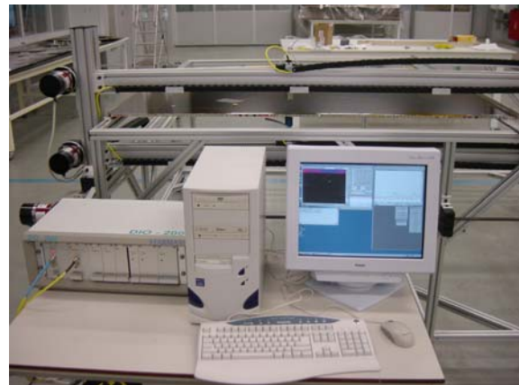
Fig. 15: Example of equipment for inspection of solar panels.
