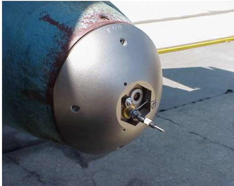
6DoF Unit installed in Nose of MK-80 Series Bomb
