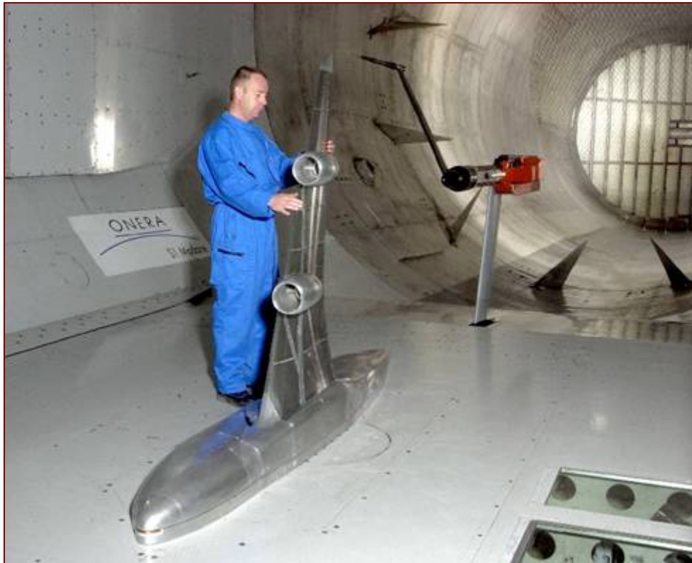
Half-model with wake traversing mechanism
