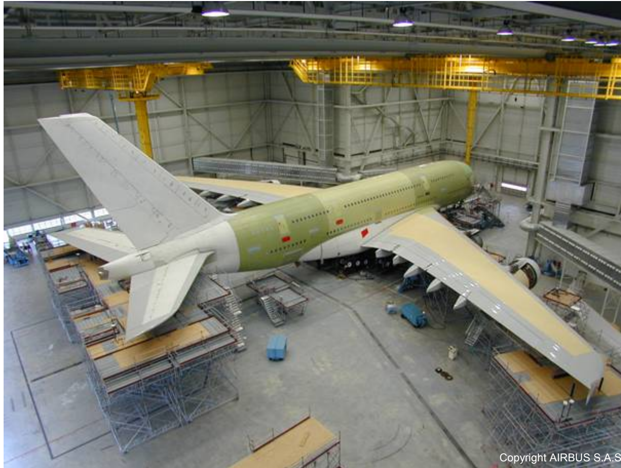
A380 during the Ground Vibration Test
