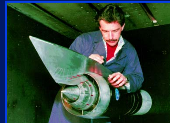
Subscale Test Model Fabricated by ASE and Installed in ASE's 5.5-Ft Transonic Wind Tunnel
