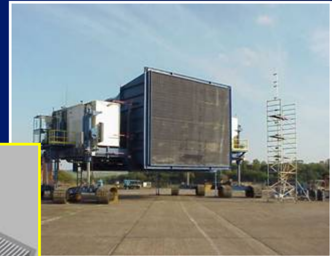
Cross Wind Blower (1,400 kg/sec at 20 to 50 knots)
