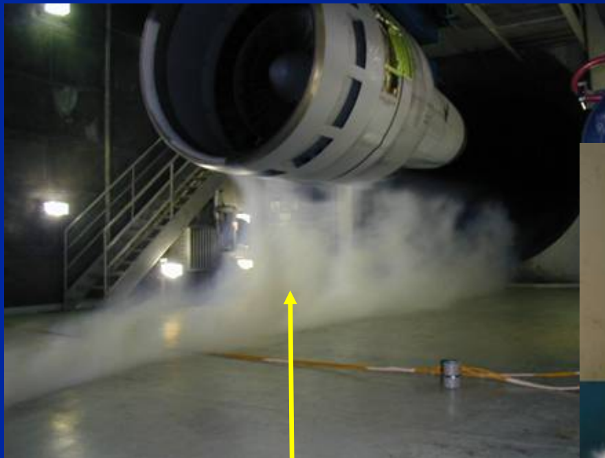
Sufficient Bypass Airflow No Recirculation Observed
