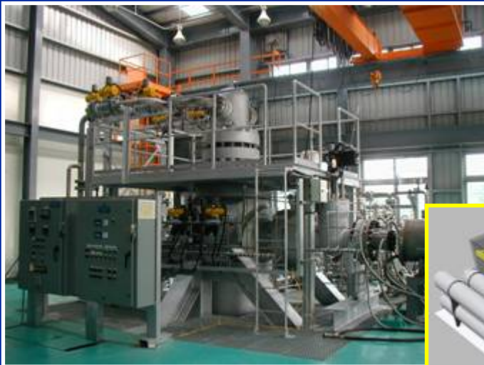
Storage Heater for Hypersonic ( P=15\text{kg/cm}^2 , 1,700k)
