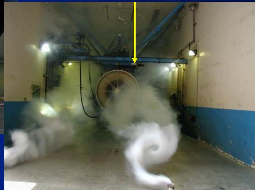
Vortex in Action Lack of Inlet Turning Device
