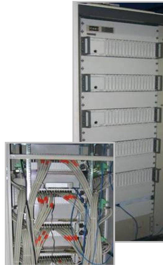
600 channel rack HBM Data Acquisition
