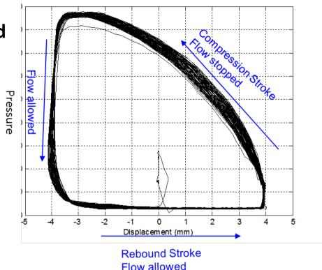
Hysteresis loop defines base component level software to control mount.
