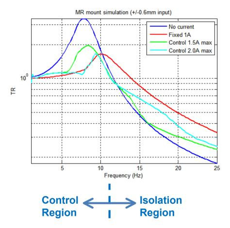
Performance can be varied by using different control algorithms and current levels.
