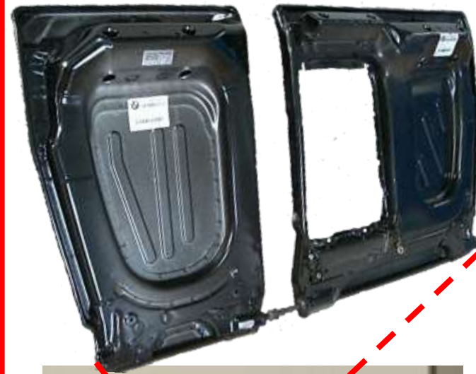
Back seat rest Steel, 12,5 kg
