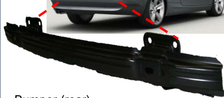
Bumper (rear) Steel, 11 kg
