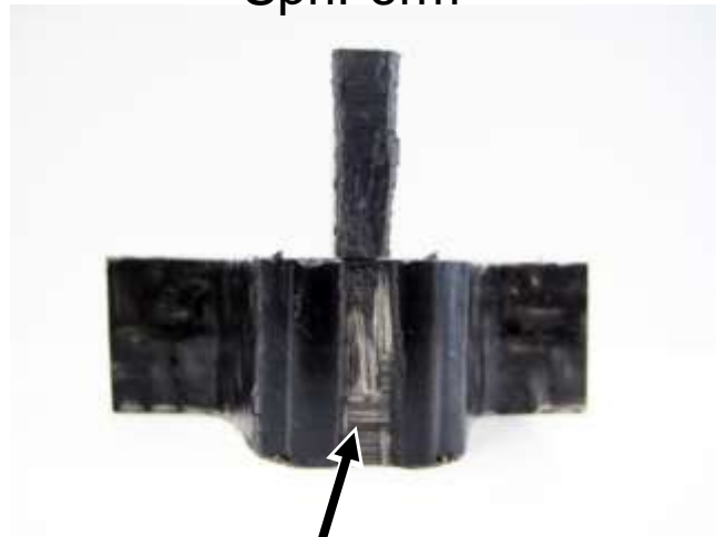
adhesion failure Spriform
