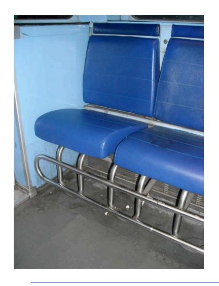
Distance holders to the heating system prevent the archiving of baggage under the seats much more than needed for security reasons
