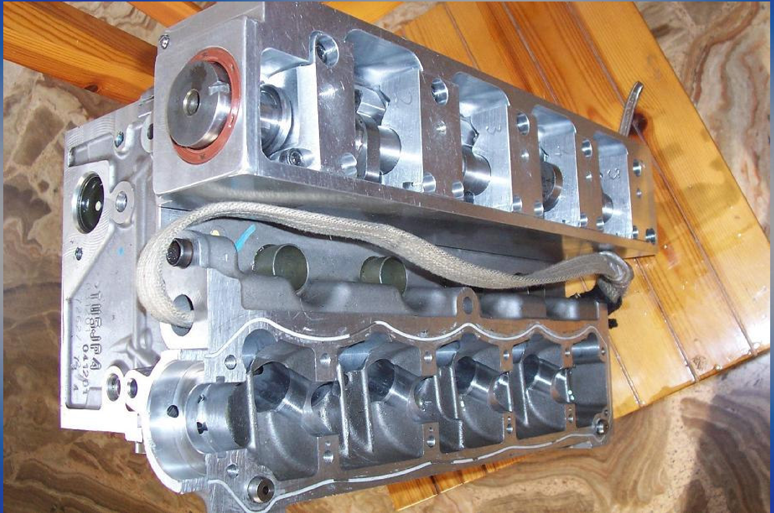
pattakon rod-roller VVA, 4cylinder, 1600cc
